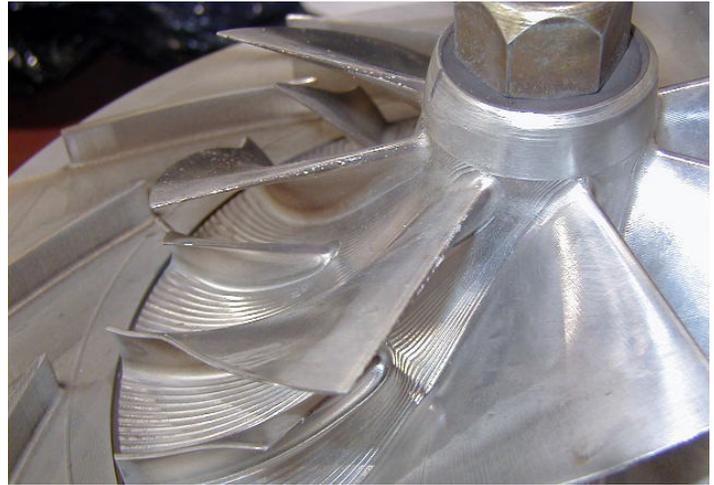
*Air end impeller installed & ready for final assembly*
