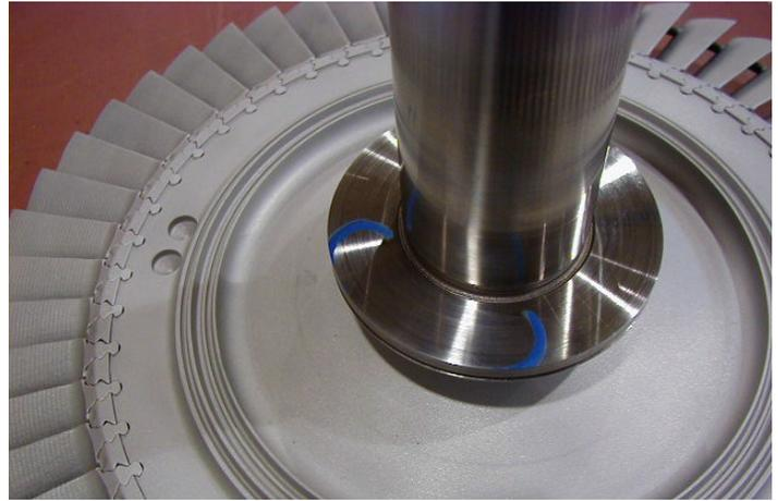
*Repaired & rebladed rotor ready for installation*
