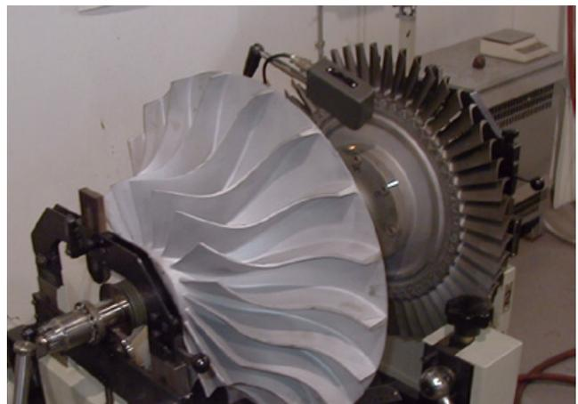
*Repaired rotor ready for balancing*
